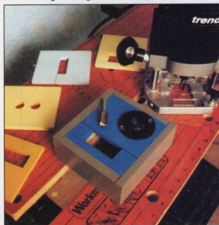
A two-piece template insert for the JKB Omni-jig
