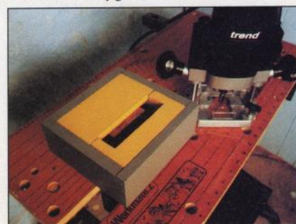
A two-piece template insert for the JKB Omni-jig
