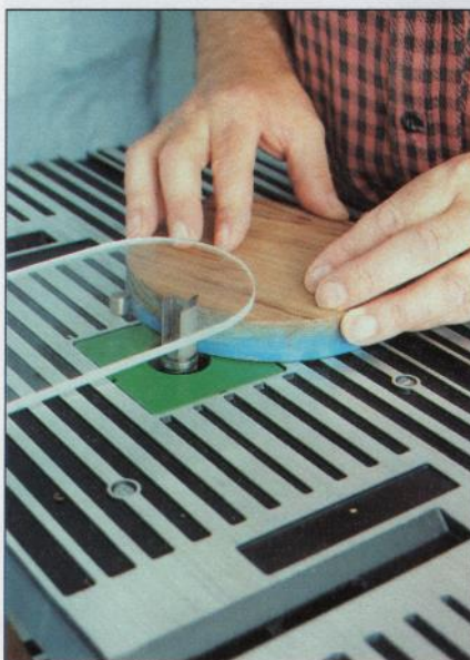
Template routing using a bearing-guided cutter. Note the lead-in pin
