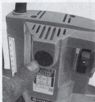
Hitachi TR8 – accessible carbon brushes
