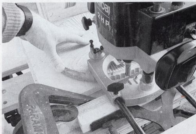
Jig for 'gear-cogging' edge of pendulum routed dish
